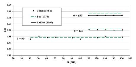
Figure 5: Discharge coefficient for the classical weir in compared to previous studies
