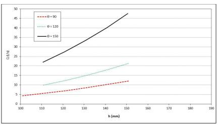
Figure 3:Relationship head-flow for classical V-notch model weirs
