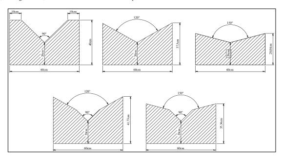
Figure 2: The tested weir models
