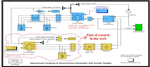
Figure 1. Simulating the synchronous generator with the exciter system
