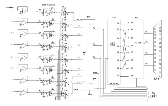
Figure 2: Circuit Diagram of Data Acquisition System
