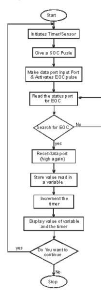
Figure 3: Flow Chart for Data Acquisition
