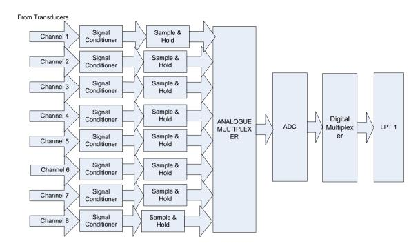
Figure 1. Block Diagram of Eight Channel Data Acquisition System
