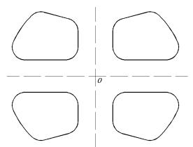
Figure 9: Typical non-slope moulds of aluminum extrusion-models
