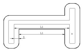
Figure 8: Offset curve along the outer contours
