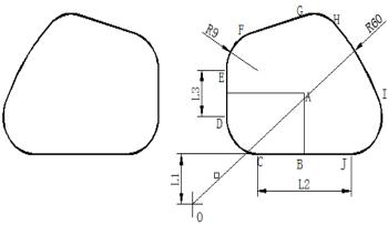
Figure 7: machining method with G91
