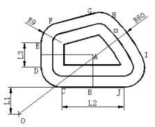
Figure 6: Circular cutting mode with start point at center
