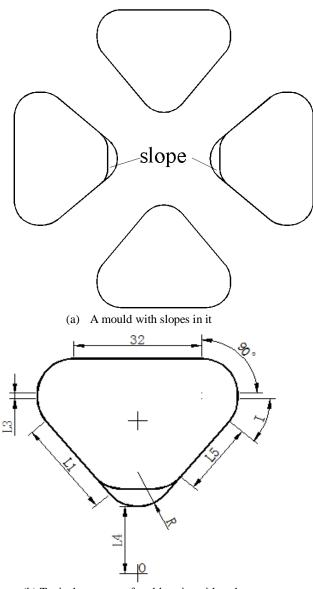
(b) Typical structure of mold cavity with a slope **Figure 11:** Mould cavity with slopes
