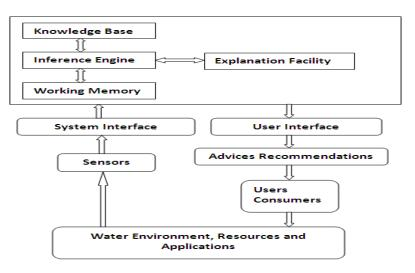
Figure 2: Structure of proposed expert system
