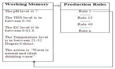
Figure 7: The production system after the Rule 1 is fired.
