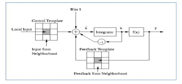
Figure 2: The Block Diagram of a CNN Cell ([1,6,7,13])
