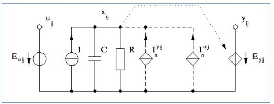
Figure 1: Circuit Representing Cellular Neural Networks ([1,6,7,13])
