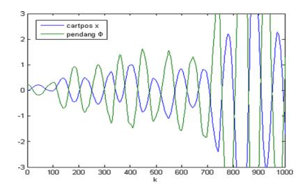
Figure 2: Open-loop response of cart position and angular position of the pendulum
