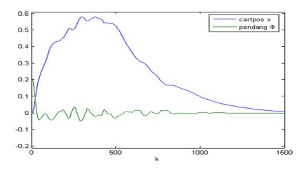
Figure 3: Closed-loop dynamic behavior of cart position and angular position of the pendulum- Case I
