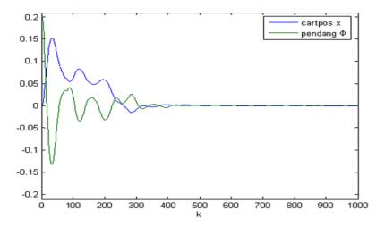
Figure 4: Closed-loop dynamic behavior of cart position and angular position of the pendulum- Case II.
