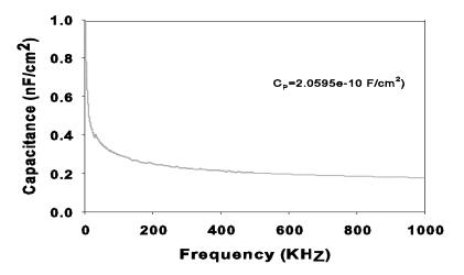
Figure 8: Device frequency versus capacitance curve
