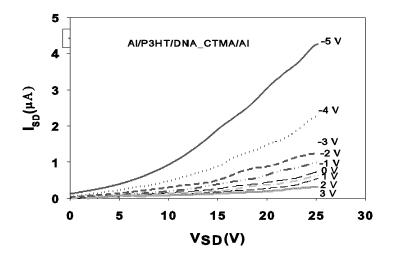
Figure 6: V<sub>SD</sub> versus I<sub>SD</sub> at different gate voltages.
