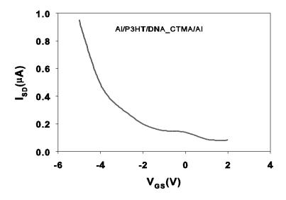
**Figure 7:** Transconductance curve at  $V_{SD}=10V$
