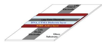
Figure 5: Fabricated device structure on glass plate
