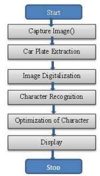
Figure 1: Flow Diagram- Process of CPR
