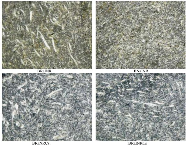
Fig.7. Abraded Surfaces of Specimens. (a) BRaNR, (b) BNaNR, (c) BRaINR, (d) BNaINR, (e) BRaCsNR, (f) BRaICsNR.
