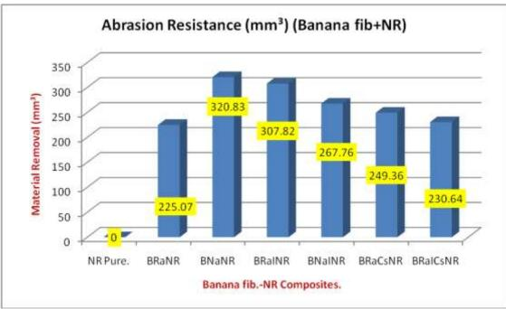
Fig.6. Wear Resistance/ Material Removal rate mm<sup>3</sup>/mm.
