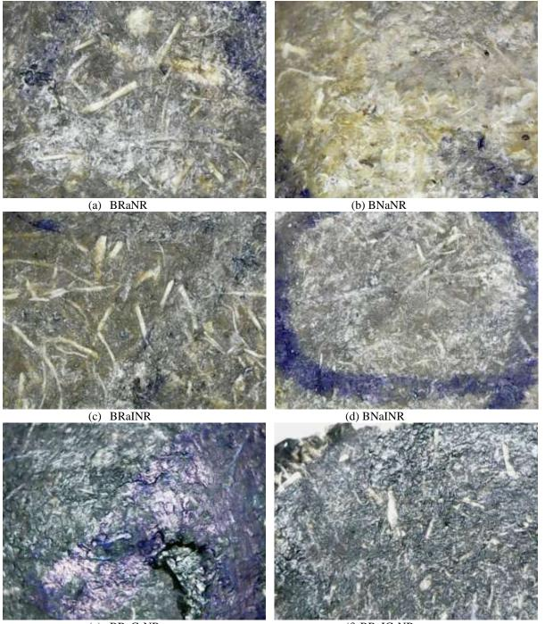
(e) BRaCsNR (f) BRaICsNR. Fig.5. Specimen Surfaces after Compression Test (a) BRaNR, (b) BNaNR, (c) BRaINR, (d) BNaINR, (e) BRaCsNR, (f) BRaICsNR.
