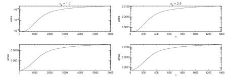
Figure 1: Plot of the root mean square of the vertical velocity (top) and the maximum velocity (bottom) with time, for  $c_p = 1.0$  and  $c_p = 2.5$ .
