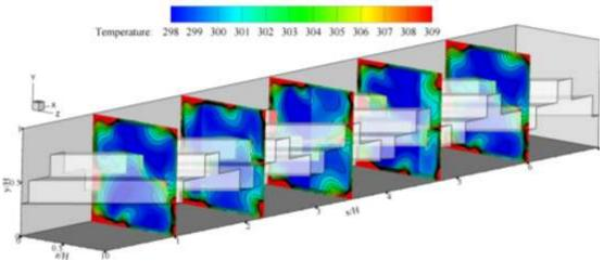
Figure 5: Temperature distributions in cross sectional planes at various positions (*x/H*) for square channel inserted with inclined wavy surface at Re = 4000 and  $\alpha = 45^{\circ}$ .
