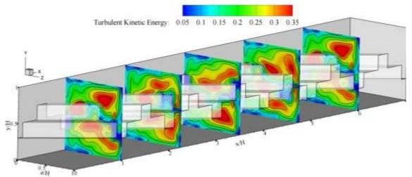
**Figure 6:** Turbulent kinetic energy (*TKE*) distributions in cross sectional planes at various positions (*x/H*) for square channel inserted with inclined wavy surface at Re = 4000 and  $\alpha = 45^{\circ}$ .
