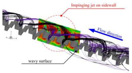
Figure 3: Impinging jet on the sidewall for square channel inserted with inclined wavy surface at Re = 4000 and  $\alpha = 45^{\circ}$ .
