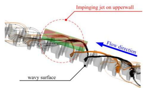
Figure 4: Impinging jet on the upper wall for square channel inserted with inclined wavy surface at Re = 4000 and  $\alpha = 45^{\circ}$ .
