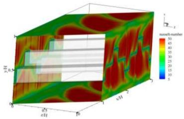
Figure 7: Local Nusselt number distributions on the channel walls for square channel inserted with inclined wavy surface at Re = 4000 and  $\alpha = 45^{\circ}$ .
