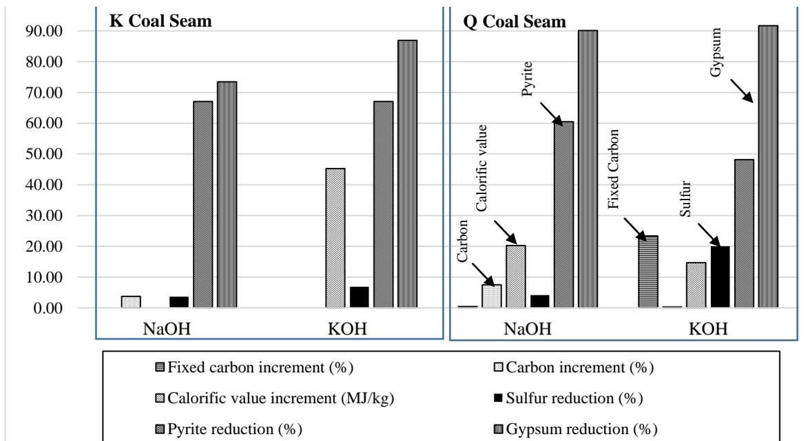
Fig. 3: The reduction and increment of the sulfur and coal quality from the K and Q coal seams in Mae Moh mine by using NaOH and KOH treatment.
